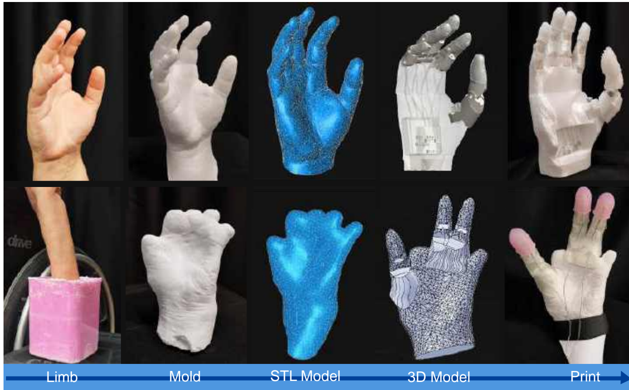
Figure S2: Five-step overview of the Human-Inspired Actuator Modeling and Reconstruction (HAMR) process applied to both a full-hand prosthetic end effector and a partial-hand fitting. The top row illustrates the HAMR workflow used to create the Tendon-Actuated Prosthetic Hand (TAPH), while the bottom row illustrates the same process applied to a flexible, 3D-printed fitting for a partial-hand prosthesis. From left to right, the steps include: (1) limb molding, (2) plaster casting, (3) 3D scanning, (4) CAD-based model reconstruction, and (5) additive manufacturing.
