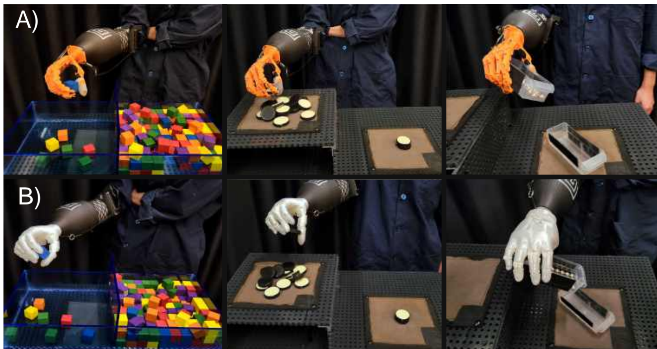
Figure 3. A participant performing the block transfer, checker transfer and stack, and carton transfer and pour tasks using (A) the BSH and (B) the TAPH end effectors.
