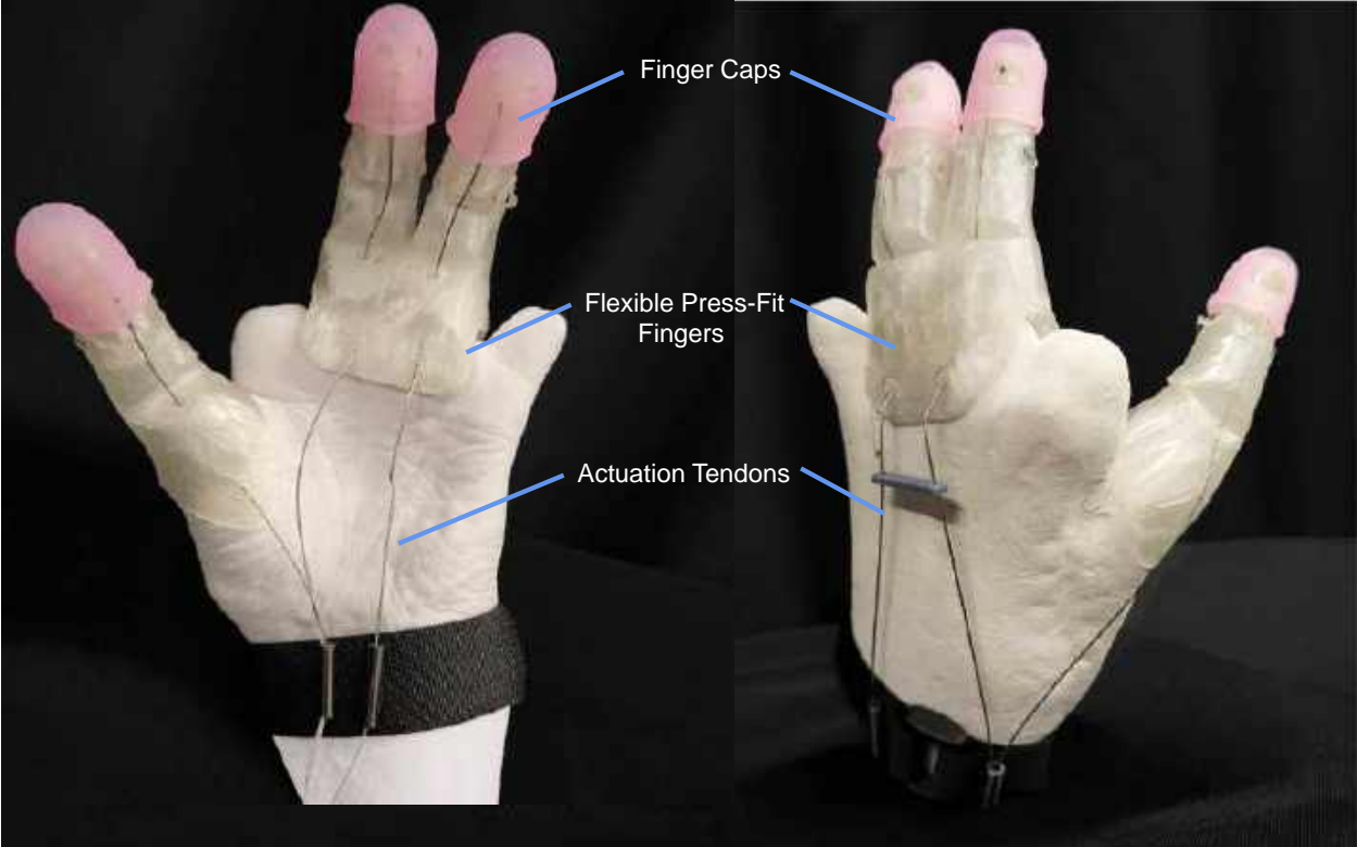
Figure S3: The multi-material custom partial hand fittings feature flexible press-fit bases, and rigid tendon-actuated finger joints.
