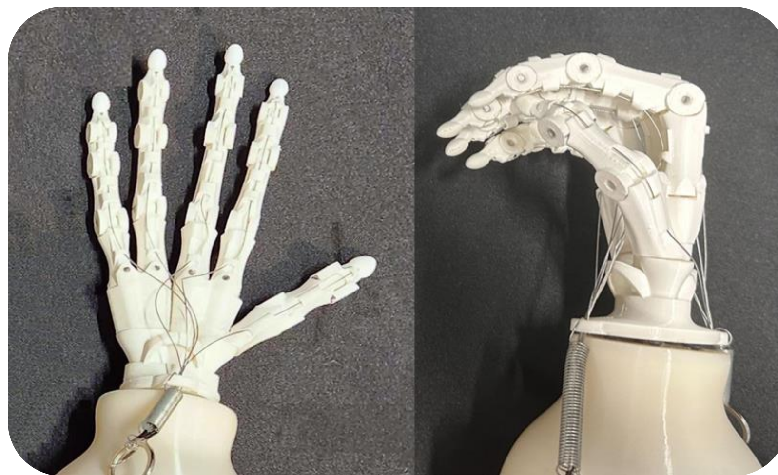
Figure 3: Original hand design in extended and grasping positions
