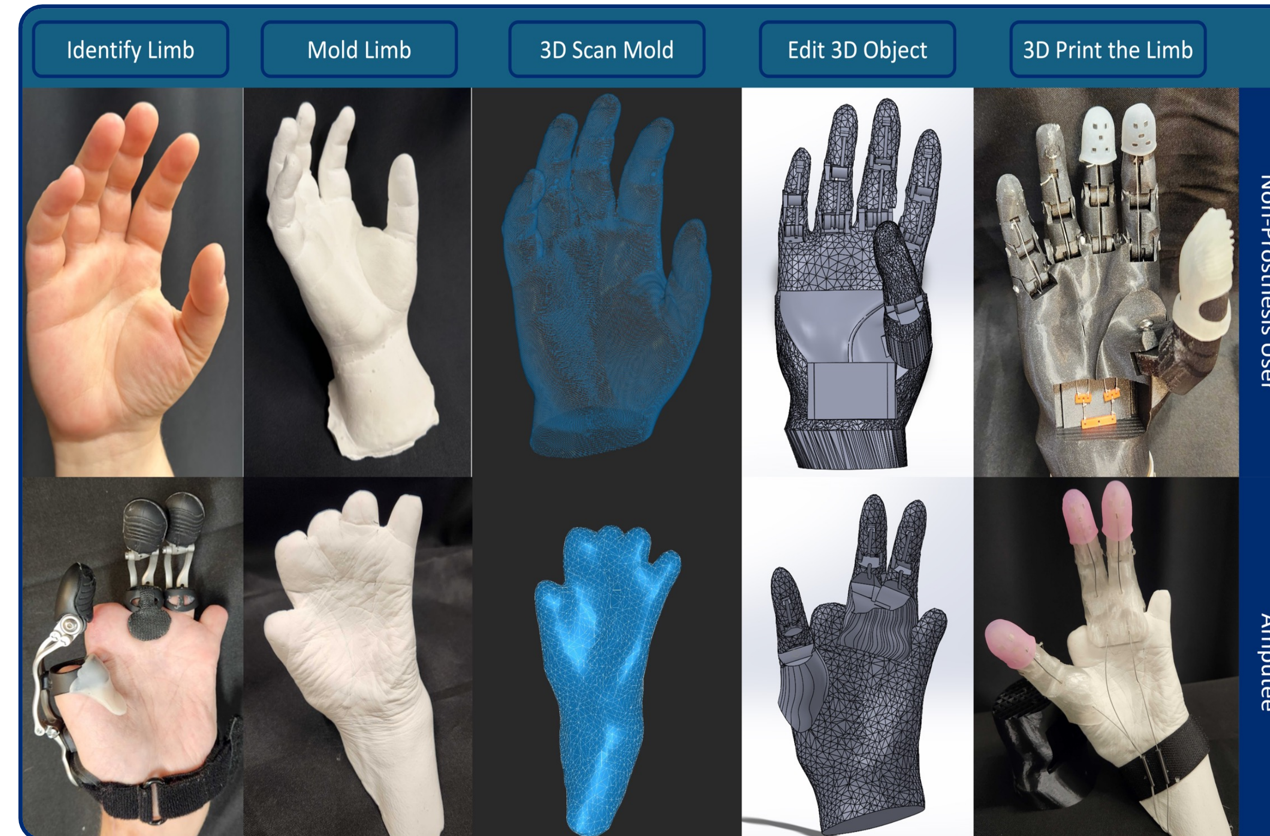
Figure 3. Process of Creating a Custom Tendon Actuated Prosthesis Hand. This figure shows a step by step process into how a prosthesis hand is created from a limb.
